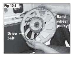
Ensure that the V grooves of the belt mate with the V grooves of the pulleys as shown in **Fig 10.6**.
